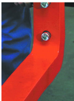
Increased forged thickness at heel of fork doubles safe life
